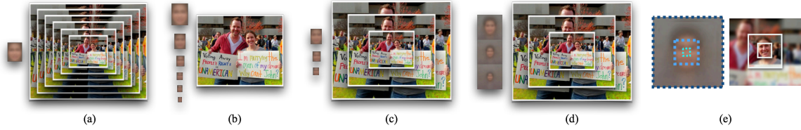
Figure 2.2: Different approaches for capturing scale-invariance. Traditional approaches build a single-scale template that is applied on a finely-discretized image pyramid (a). To exploit different cues available at different resolutions, one could build different detectors for different object scales (b). Such an approach may fail on extreme object scales that are rarely observed in training (or pre-training) data. We make use of a coarse image pyramid to capture extreme scale challenges in (c). Finally, to improve performance on small faces, we model additional context, which is efficiently implemented as a fixed-size receptive field across all scale-specific templates (d). We define templates over features extracted from multiple layers of a deep model, which is analogous to foveal descriptors (e).
